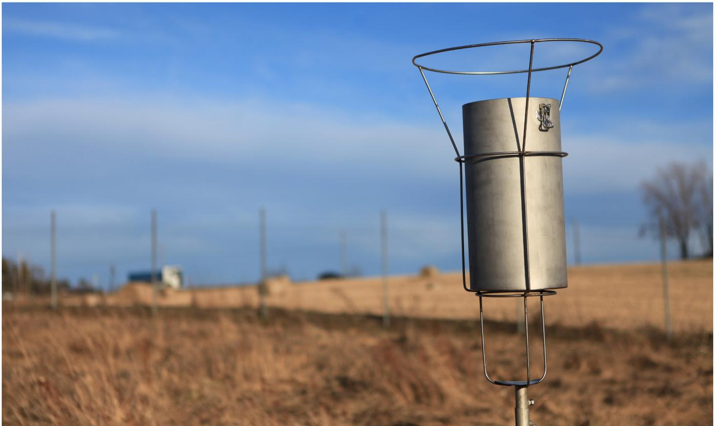
The stainless-steel collector is designed to minimize contamination of the sample and when preparing the sampler for field measurements are heated to more than 400° C to make sure the sampler is clean. The Atmospheric Microplastic Collector can be used in parallel with a precipitation sampler if the amount of precipitation is important.
